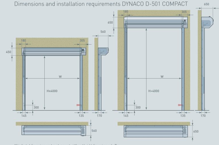
All indicated dimensions are based on exact width and height dimensions only. The space necessary for mounting and maintenance has to be provided.
