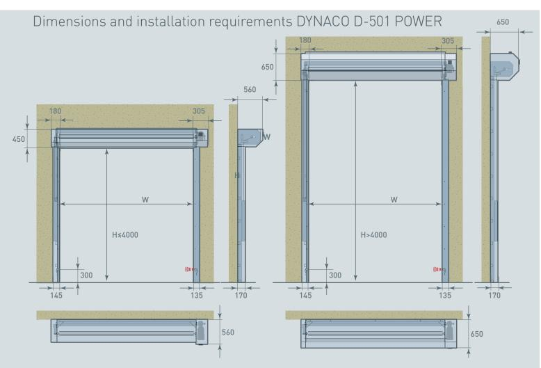
All indicated dimensions are net: the space necessary for mounting and maintenance has to be provided.
