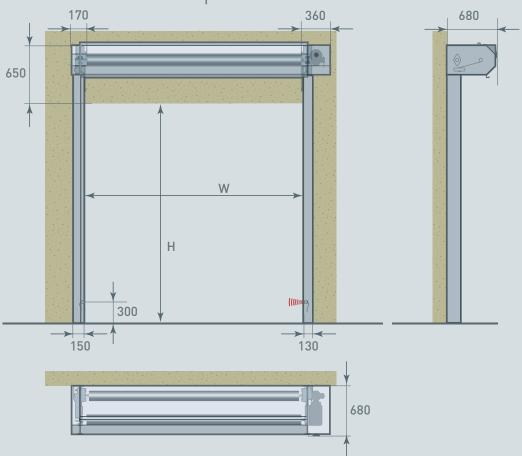
All indicated dimensions are net: the space necessary for mounting and maintenance has to be provided. Remark: drum cover available for doors up to 5900mm
